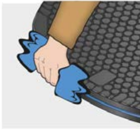
Cover seals and seating faces should be cleaned with a damp microfibre cloth.
