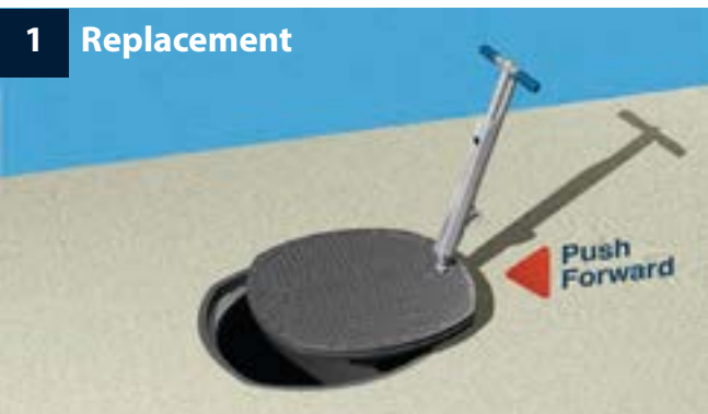
Push back the cover into the frame with the aid of the lifting tool and your foot if necessary. Step down on the cover to re engage the seal.
