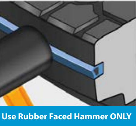
Ensuring correct orientation. Taking care, 'gently' tap new seal into position.
