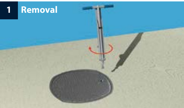
Insert the lifting tool into the lock aperture as shown above and turn the handle through 90° clockwise towards you.
