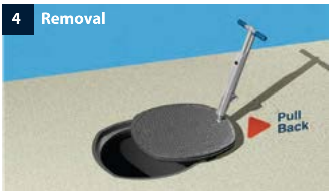
Fold back the seal breaker into the lifting tool. Lift the edge of the cover until free of frame. Pull the cover out of the frame.
