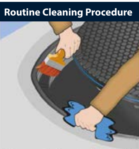
The frame seating face should be brushed and cleaned every time the cover is lifted.
